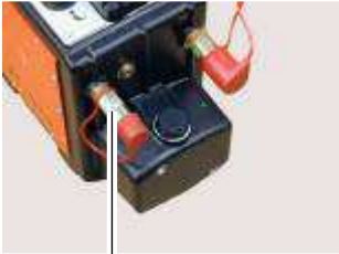
Oil tank ECO1, ECO2
